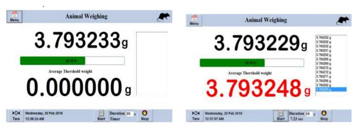
Once it is completed the above reading will show you the normal weighing reading and the bellow reading will freeze animal average Threshold weight reading.
