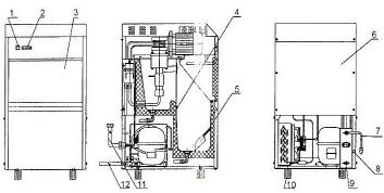
1. Switch 5. Ice Shovel Outlet 9. Water 2. Operation Board 6. Back Panel Tube 3. Door 7. Power Cable 10. Foot Screw Temperature 8. Screw for 11. Water Inlet Tube Sensor Drainage
