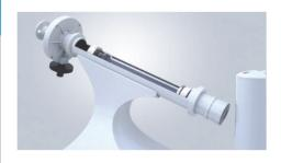
Rotate the vernier knob till the visual field to equal brightness. (Zero point)
