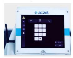
Possibility of saving 100 different types of welding programs with different parameters, make it easy for welder not required to remember for dynamic need of parameter depending upon type of metal.
