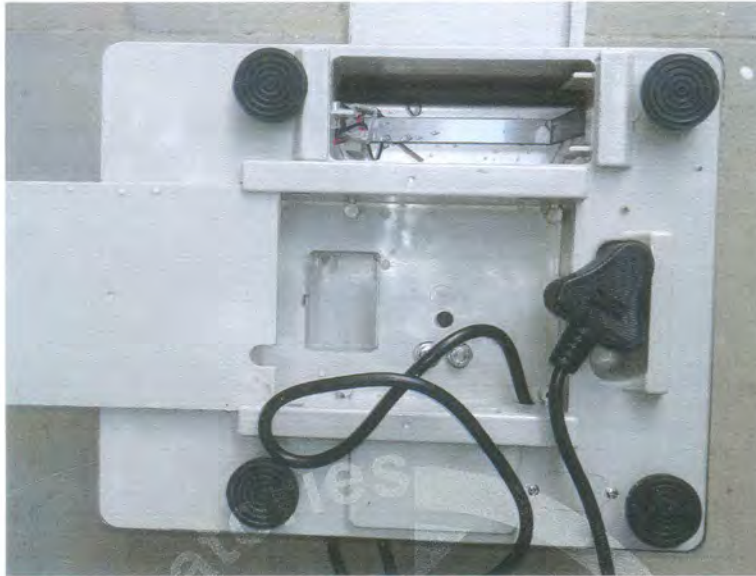
Picture3: Ingress of water (18 ml) observed
