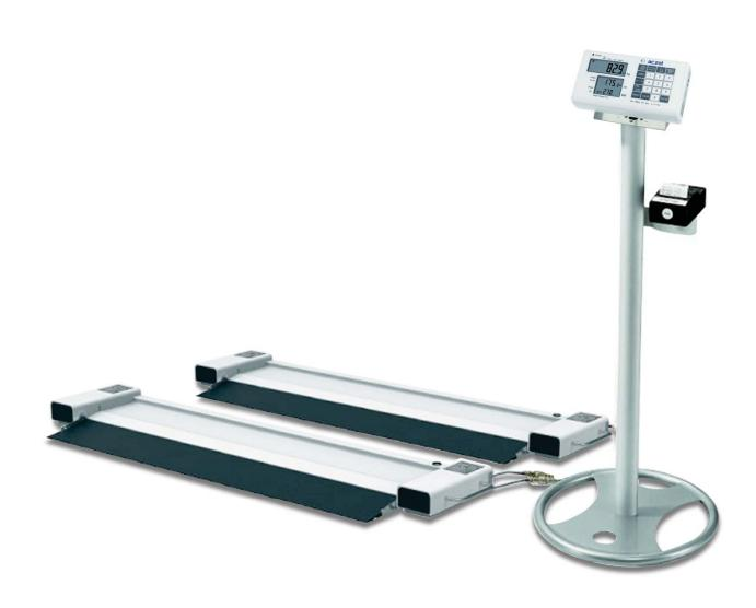
Scales designed for weighing patients in lying position. The construction of bed scales allows to use of any kind of bed with various braking systems. Due to long weighing beams the measurement of bed mass can be performed in any place on the beams. The beams can be extended up to 2,5 meter for all possible dimensions of beds. The scale's measuring indicator is equipped with LCD display, powered either from mains or from batteries.
